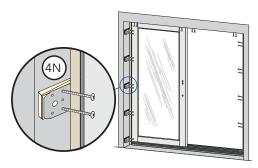
O. Drive #10 x 3-1/2" corrosion resistant wood screws through the holes in the threshold in to the floor.
